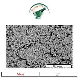
Fig. 2. Fragments of microstructure of ceramics of SS of the system (1-x) BaTiO<sub>3</sub>- xSrTiO<sub>3</sub> in the interval  $0.0 \le x \le 1.0$  (Figure shows values of x).
