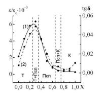
Fig. 5. Relationships of relative dielectric permeability,  $\epsilon/\epsilon_0(1)$ , dielectric dissipation factor tg $\delta$  (2) TP (1-x) BaTiO<sub>3</sub>-xSrTiO<sub>3</sub> and concentration of SrTiO<sub>3</sub>.
